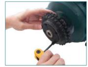
**REMOVING A TAPER LOCK BUSH**
